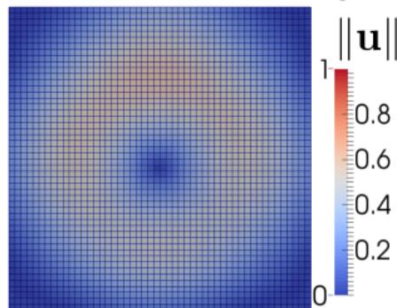
$\kappa_{ij} = 0$  (LM) and  $\kappa_{ij} = \min\left(1, \frac{|u_{ij}|}{c_{ij}}\right)$  (AM) on a cartesian  $50 \times 50$  :
