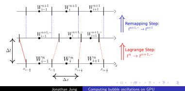
Equations Lagrangian step Remapping step Properties of the scheme
