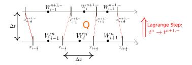
The integration of  $\partial_t W + \partial_x F(W) = 0$  on the space-time quadrilateral Q gives:
